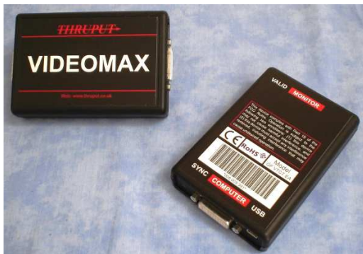
The Thruput VIDEOMAX Graphics Accelerator enables PCoIP portals, Thin clients or HDMI equipped laptops to drive high-resolution monitors and projectors
