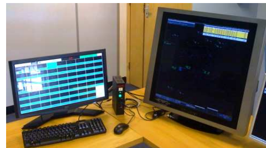
A dual output PCoIP portal from ClearCube is shown driving a 28" 2048 x 2048 monitor using Videomax as well as a 27" 1920 x 1200 touch screen.
