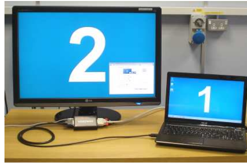
In this photograph an ASUS laptop is connected by VIDEOMAX to an LG 30" 2560 x 1600. The display manager identifies each of the screens.
