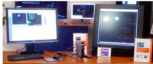
A dual output PCoIP portal from EVGA is shown driving both 28" 2048 x 2048 and 30" 2560 x 1600 monitors using Videomax.
