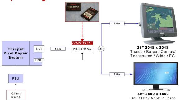
Thruput Pixel Repair (and Colour Calibration) Systems are compatible with any monitor resolution and are wholly independent of the data source.
