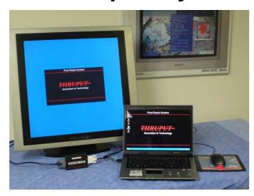
The Thruput Pixel Repair System is a tool for restoration of normal operation to monitors that have developed a ghosted image, or frozen pixels during their operational life.
