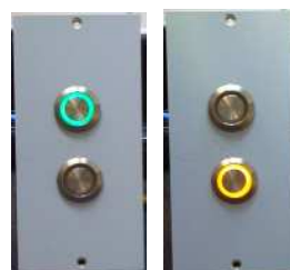
Figure 3 Top left: The console mounted switch of the GF 1030 SW has colour coded, console mounted switches:
