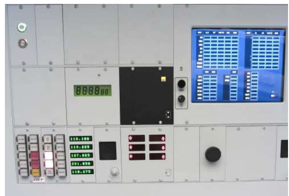
Figure 3 Top left: The console mounted switch of the GF 1030 SW has colour coded, console mounted switches:
