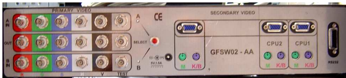
Below: Front panel showing the Sony DDM interfaces (left) and conventional Keyboard, Mouse and Video interfaces (right)
