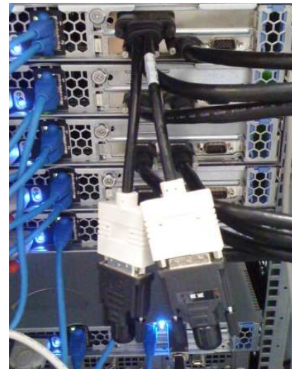
Thruput DVI dummy monitor is deployed at Warsaw ACC to provide remote real time monitoring of 2048 x 2048 Air Traffic Control positions.
