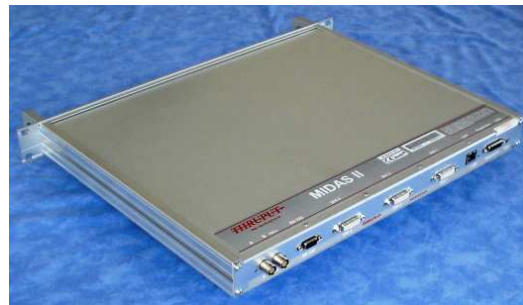
Merlin helicopter: MIDAS 2 Video processing Unit.
