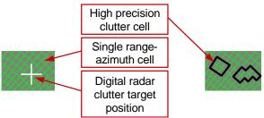
The high speed of FPGA logic enables an unlimited number of high precision clutter cells to be defined. In this example they are the range-azimuth cells affected by two clutter sources: An individual wind turbine and the traffic on a road bridge.
