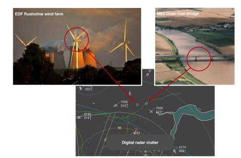
All primary Radars perceive the world in terms of range and azimuth cells, which, in modern radars, are then digitally processed for display to Air Traffic Controller's.
