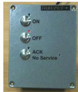
Left: The MIDAS hardware is a rack mount unit that fits in the ATC console. The photograph shows its dual redundant power supplies and universally standard video interfaces. Right: MIDAS clutter reduction indicator panel.
