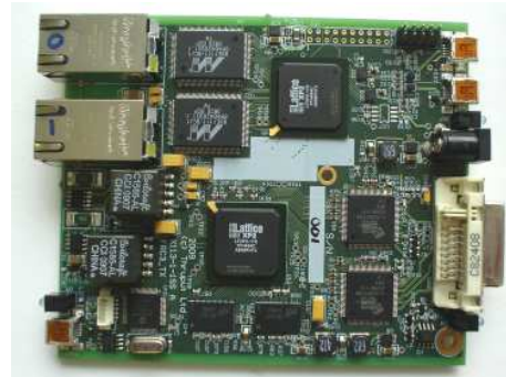
Sentinel Tx uses high-performance, low-power FPGA technology
